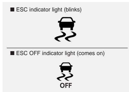
When the POWER button is pressed to the ON position, the ESC indicator light illuminates, then goes off if the ESC system is operating normally.
