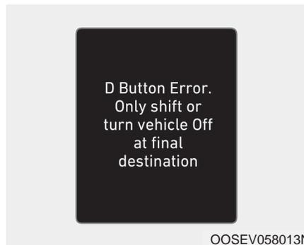
The message is displayed when there is a problem with the D button. If this message is displayed, do not shift the gear or turn the vehicle off while driving. If the driver shifts the gear to P/R/N position or turns off the engine, it is impossible to shift back to D (Drive).
