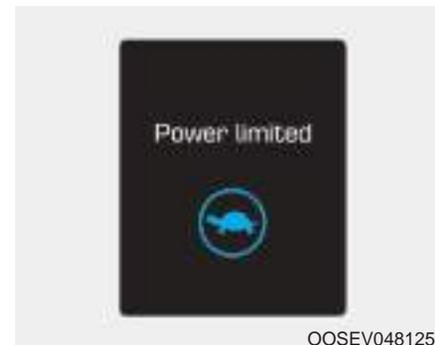
In the following cases, this warning message is displayed when the vehicle's power is limited for safety.
