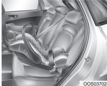
A rearward-facing child seat provides restraint with the seating surface against the back of the child. The harness system holds the child in place, and in an accident, acts to keep the child positioned in the seat and reduce the stress to the neck and spinal cord.
