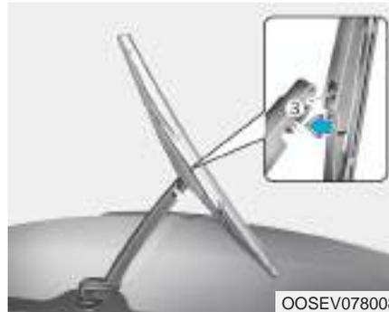
3. Install the new blade assembly by inserting the center part into the slot in the wiper arm until it clicks into place (3).
