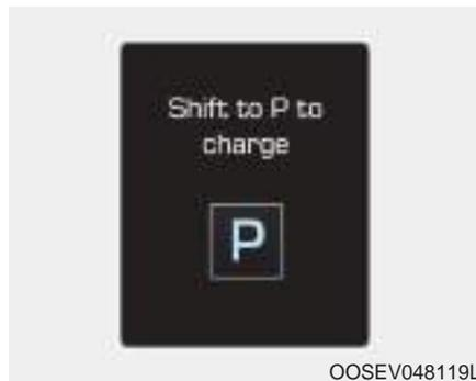
This message is displayed if you connect the charging cable without the gear in the P (Park) position. Shift to P (Park) before connecting the charging cable.
