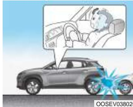
Front air bags are not designed to inflate in rear collisions, because occupants are moved backward by the force of the impact. In this case, inflated air bags would not provide any additional benefit.
