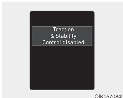
Press and hold the ESC OFF button continuously for more than 3 seconds. The ESC OFF indicator light and message "Traction & Stability Control disabled" illuminates and a warning chime sounds. In this state, both the traction control function of ESC and the brake control function of ESC are disabled.
