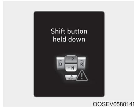
The message appears on the LCD display when the shift button is continuously pressed or there is problem with the button.
