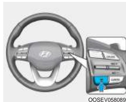
When Smart Cruise Control system is ON, you can set and maintain the distance from the vehicle ahead of you without pressing the accelerator or brake pedal.
