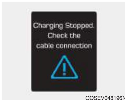
This warning message is displayed when charging is stopped because the charging connector is not correctly connected to the vehicle charging port.
