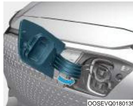
1. After recharging, make sure to install the charging port dust cover(s) before closing the charging door.
