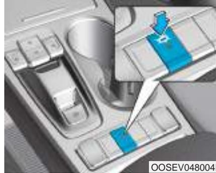
When the POWER button is in the ON position or when the vehicle is in the ready (🚗) mode, press the heated steering wheel button to warm the steering wheel. The indicator on the button will illuminate.
