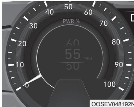
The torque gauge shows the real-time torque value while driving when SPORT mode is selected by pressing the DRIVE MODE button.
