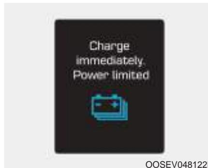
When the high voltage battery level reaches below 3%, this warning message is displayed.
