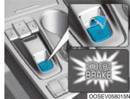
**To apply the EPB (Electronic Parking Brake):**
