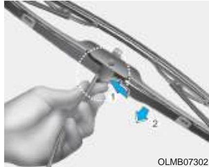
2. Press the clip (1) and slide the blade assembly downward (2).
