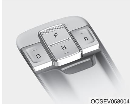
Select the desired gear by pressing one of the buttons on the Gear Shift Selector.
