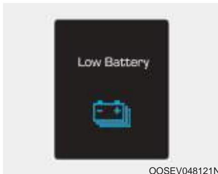
When the high voltage battery level reaches below 8%, this warning message is displayed.
