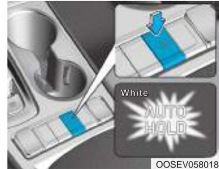
1. With the driver's door, hood and liftgate closed, depress the brake pedal and then press the [AUTO HOLD] switch. The white AUTO HOLD indicator will come on and the system will be in the standby position.
