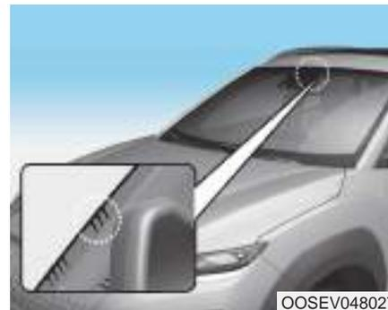
Auto defogging helps reduce the possibility of fogging up the inside of the windshield by automatically sensing the moisture on inside the windshield. The auto defogging system operates when the heater or air conditioning is on.
