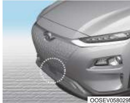
Smart Cruise Control uses a sensor to detect distance to the vehicle ahead.
