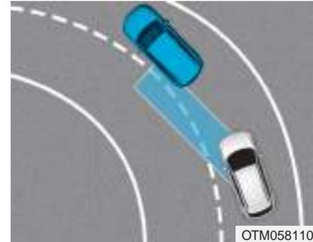
The BCW and BCA systems may not operate properly when driving on a curved road. In certain instances, the system may recognize a vehicle in the same lane.
