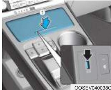
You can use a USB cable to connect audio devices to the vehicle USB port.
