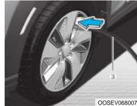
3. Connect the other end of the filling hose (3) directly into the tire valve.
