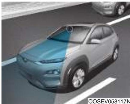
Lane Keeping Assist system helps detect lane markers on the road with a camera at the front windshield, and assists the driver's steering to help keep the vehicle between lanes.
