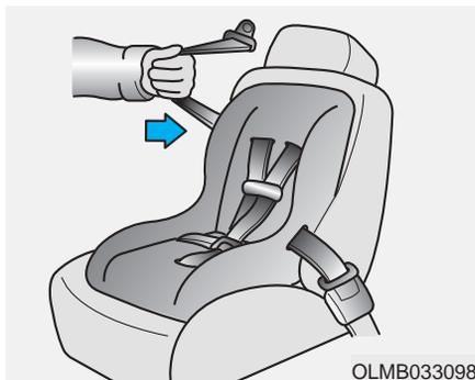
5. Slowly allow the shoulder portion of the seat belt to retract and listen for an audible "clicking" or "ratcheting" sound. This indicates that the retractor is in the "Automatic Locking" mode. If no distinct sound is heard, repeat steps 3 and 4.
