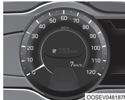
The sub speedometer is displayed on the cluster when you select ‘Other features → Speedometer subscale’ in the User Settings mode. The sub speedometer is not displayed if you deselect it in the User Setting mode.
