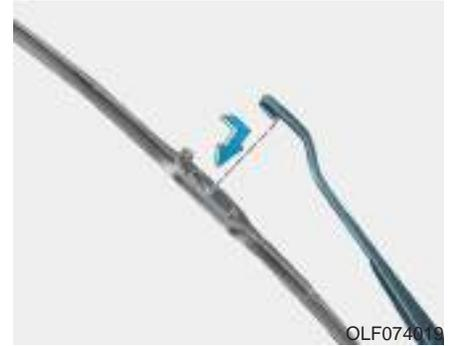
3. Install a new wiper blade assembly in the reverse order of removal.
