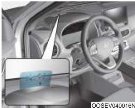
The Head-Up Display is an optional feature that allows the driver to view information projected onto a transparent screen while still keeping your eyes safely on the road ahead while driving.
