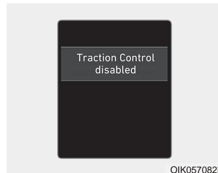
Press the ESC OFF button briefly. The ESC OFF indicator light and message "Traction Control disabled" will illuminate. In this state, the traction control function of ESC is disabled, but the brake control function of ESC still operates.
