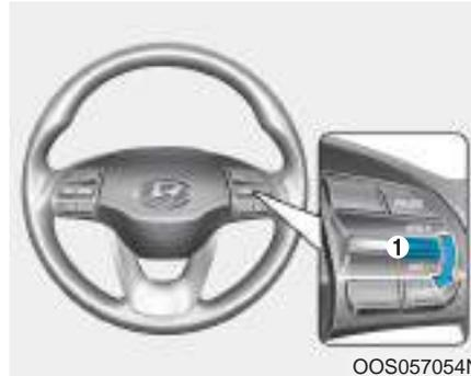
3. Push the switch (1) down (SET-), and release it. The set speed on the LCD display will illuminate.
