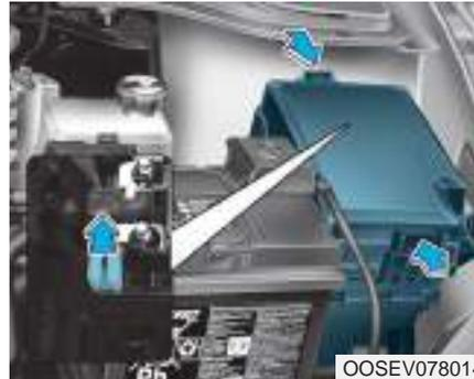
5. Pull the suspected fuse straight out. Use the removal tool provided in the motor compartment fuse panel.
