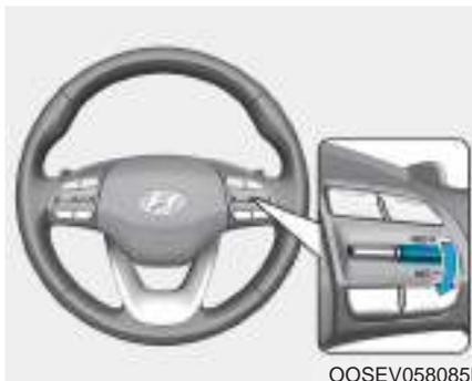
3. Push the switch down (SET-). The Set Speed and Vehicle-to-Vehicle Distance on the LCD display will illuminate.
