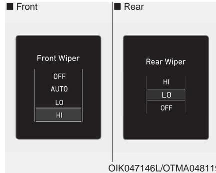
This indicator displays the windshield wiper mode when selected using the windshield wiper stalk.
