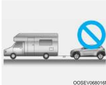
Your vehicle is not designed to be flat-towed behind a motor home. To avoid serious damage to your vehicle, do not flat-tow your vehicle.
