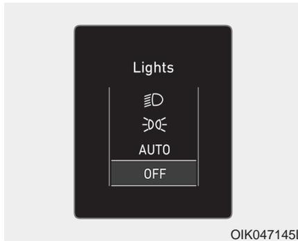
This indicator displays the exterior lights mode when selected using the headlamp control stalk.
