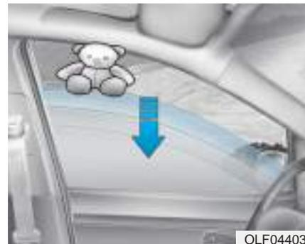
If a window senses any obstacle while it is closing automatically, it will stop and lower approximately 12 inches (30 cm) to allow the object to be cleared.
