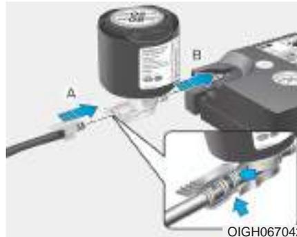
2. Connect the filling hose (3) to the sealant bottle (2) in the direction of (A) and connect the sealant bottle to the compressor (5) in the direction of (B).
