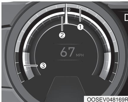
When ECO mode or ECO+ mode (if equipped) is enabled, the speedometer display includes a Smart ECO Pedal Indicator. The indicator encourages efficient driving by displaying the desired acceleration to achieve optimum range efficiency.
