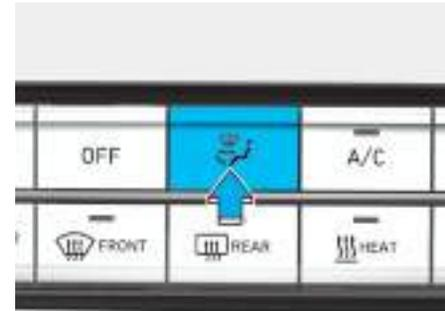
The mode selection button controls the direction of the air flow through the ventilation system.
