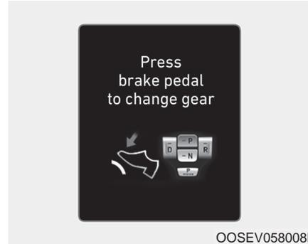
The message appears on the LCD display, when the brake pedal is not depressed while shifting the gear. Depress the brake pedal and then shift the gear.
