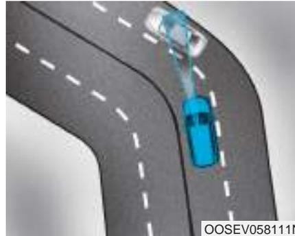
Forward Collision-Avoidance Assist system may recognize a vehicle in the next lane or outside the lane when driving on a curved road.
