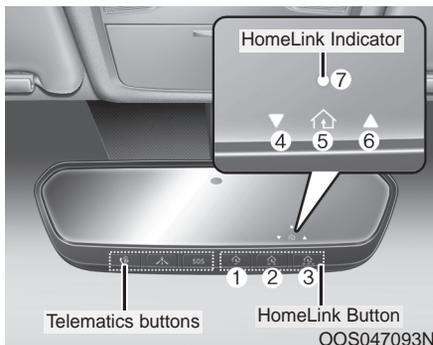
Your vehicle may be equipped with a Gentex Automatic-Dimming Mirror with a Z-Nav™ Electronic Compass Display and an Integrated HomeLink® Wireless Control System. During nighttime driving, this feature will automatically detect and reduce rearview mirror glare while the compass indicates the direction the vehicle is traveling. The HomeLink® Universal Transceiver allows you to activate your garage door(s), electric gate, home lighting, etc.
