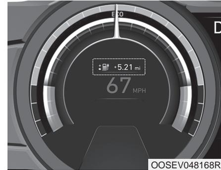
When ECO mode or ECO+ mode (if equipped) is enabled, the speedometer display includes an additional range value which is accumulated as a result of regenerative braking. The value starts from zero and incrementally increases as the energy from regen braking increases. The display resets to zero when the regen level drops to zero (vehicle accelerating, etc.).
