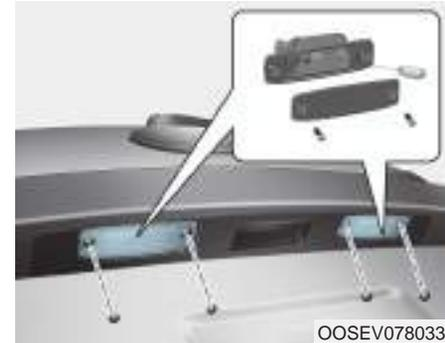
1. Loosen the lens retaining screws with a cross-tip screwdriver.
