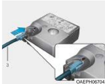
2. Connect the filling hose (3) directly into the compressor.
