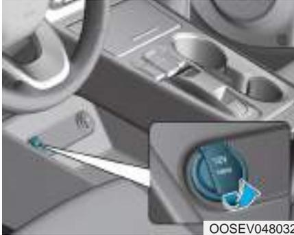
The power outlet is designed to provide power for 12V accessories or other devices designed to operate with vehicle electrical systems. The devices should draw less than 180 W with the vehicle in the ready (🚗) mode.
