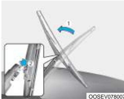
1. Raise the wiper arm and then rotate the wiper blade assembly (1).
