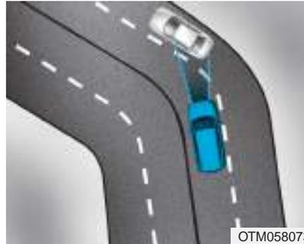
Your vehicle speed can be reduced due to a vehicle in the adjacent lane. Apply the accelerator pedal and select the appropriate speed. Check to be sure that the road conditions permit safe operation of the Smart Regeneration System.
