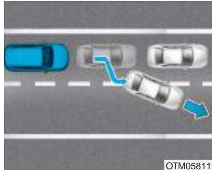
When driving in stop-and-go traffic, and a vehicle in front of you merges out of the lane, the FCA system may not immediately detect the new vehicle that is now in front of you. In this case, you must maintain a safe braking distance, and if necessary, depress the brake pedal to reduce your driving speed in order to maintain a safe distance.
