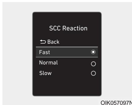
The sensitivity of vehicle speed when following the front vehicle to maintain the set distance can be adjusted. Go to the 'User Settings → Driver Assistance → SCC Reaction → Fast/Normal/Slow' on the LCD display. You may select one of the three stages you prefer.
