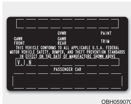
The certification label is located on the driver's door sill at the center pillar and shows the maximum allowable weight of the fully loaded vehicle. This is called the GVWR (Gross Vehicle Weight Rating). The GVWR includes the weight of the vehicle, all occupants, fuel and cargo.
